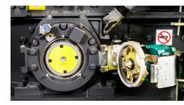
Patented rotor locking and positioning device for increased safety
