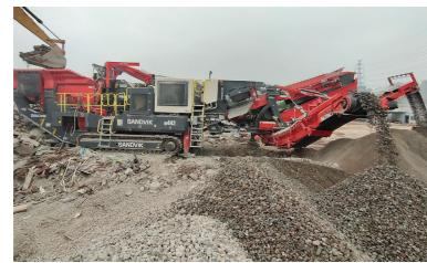
Featuring Sandvik's unique Cl621 Prisec impact chamber (5 patents pending). The Prisec concept enables one base crusher to be configured as either a Primary or Secondary chamber whilst maintaining optimum crushing geometry.
