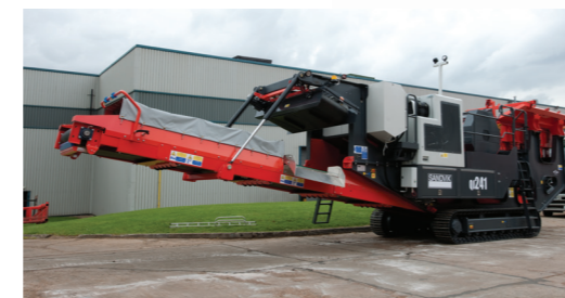
Hydraulic raise and lower facility
