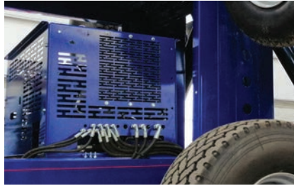
Electric Hydraulic Power pack - 11Kw & 30Kw (Set Up Functions only)
