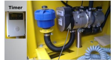
HEATING SYSTEM FOR ENGINE
