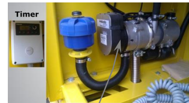
HEATING SYSTEM FOR ENGINE
