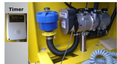
HEATING SYSTEM FOR ENGINE
