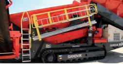
Hydraulically folding maintenance platforms
