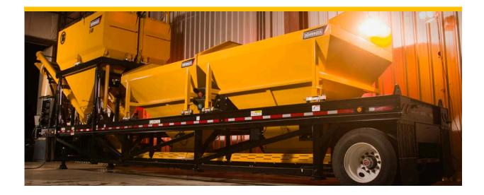
The 6<sup>th</sup> generation B-100 concrete batch plant is designed and built to Böhringer's exacting standards, delivering first in class versatility and performance – with achievable batching times of 2-3 minutes per cycle\*.
