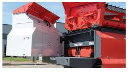
Hydraulically opening powerpack for ease of maintenance Hydraulically folding doors for easy access
