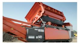
Tipping function activated by radio remote control
