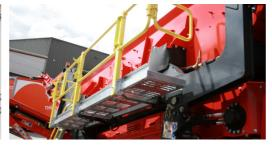
Hydraulically folding maintenance platforms
