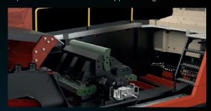
Includes integrated lifting jib, chain hoist and lifting cradle for safe removal, rotation and fitment of hammers
