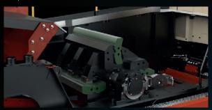
Unique 4 key trapped system to ensure safe inspection after the rotor has stopped turning
