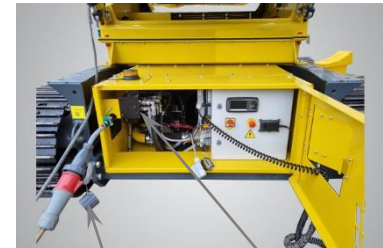
Hydraulic pump with E-motor
