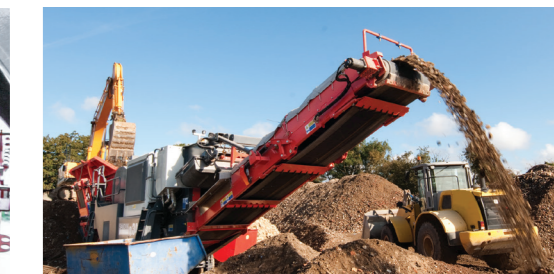
Long main conveyor for massive stockpiling
