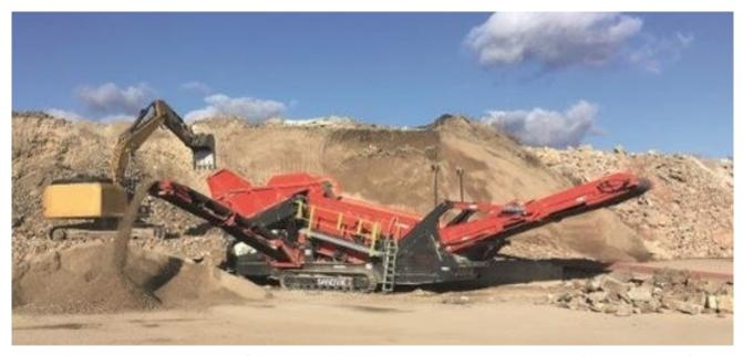
The new Sandvik QE342 is an evolution of the class leading Sandvik QE341 which comes with a host of updates and new features. The Sandvik QE342 is a heavy duty scalper with class leading open scalping area enabling it to deliver enormous rates of production.
