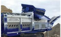
Twin Deck Vibrating Grid - Available with remote tipping function.
