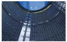
Mesh Panels - A large screening are suitable for compost, mulch, topsoil etc.
