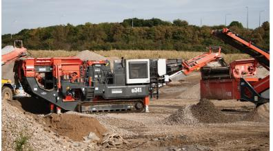
Featuring Sandvik's unique Cl611 Prisec impact chamber (5 patents pending). The Prisec concept enables one base crusher to be configured as either a Primary or Secondary chamber whilst maintaining optimum crushing geometry.
