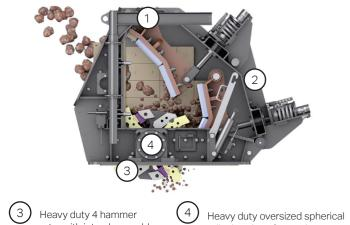
rotor with interchangeable hammer configuration.
